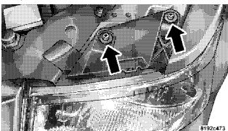
2. Remove one nut that attaches the headlight to the inner fender panel. Access to the nut is possible by opening the fender panel access door which is located in the wheel liner.
